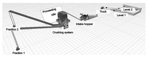
Fig. 1. 3D view of schematic production system in mineral aggregates mine
